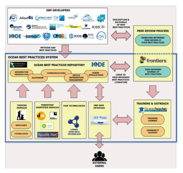
OBPS structure (large box across middle of figure), core technologies (along the bottom of the box), and best practice provider organizations (in the box at top). Training is shown at the bottom right.(Pearlman et al., 2021)
