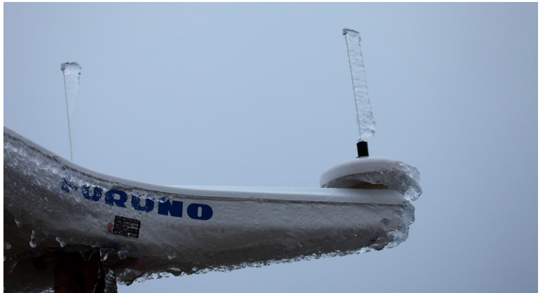
Figure 7.1: Ice accretion on a GPS compass scanner. Courtesy of Shell
