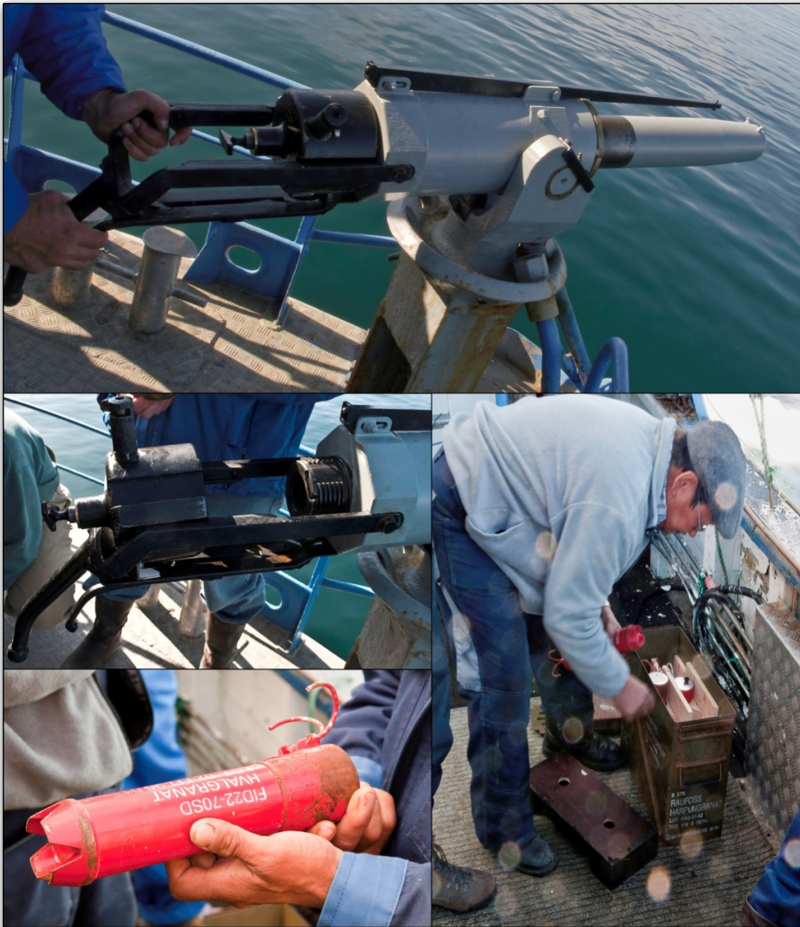
Plate III. Examples of harpoon cannon and whale-grenades in Greenland. (Photo: Greg Donovan).
